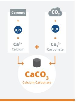
$CO_2$  mineralization uses waste  $CO_2$  in concrete production. In this process  $CO_2$  is converted to a solid mineral (calcium carbonate), permanently removing these emissions from the atmosphere.
