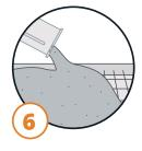
Once injected, the CO<sub>2</sub> converts into a nano-sized mineral that becomes permanently embedded in the concrete.
